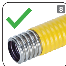
After 5 waves / corrugations are undressed
