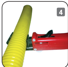
Cutting the hose by apparatus and undressing the outer coating. Can the coating be undressed first, then the cutting shall also be performed.
