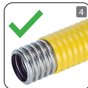
Ensure that five corrugations are intact and undamaged prior to installation.
